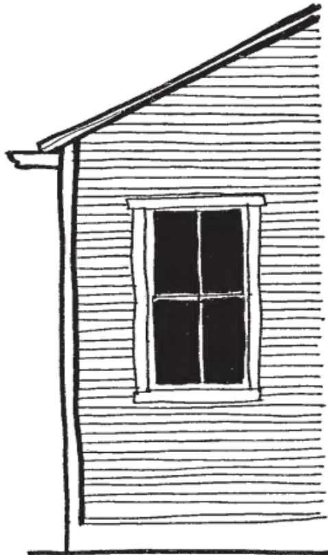
Appropriate: Narrow siding is properly in scale. Preserves corner, sill, and window trim.
