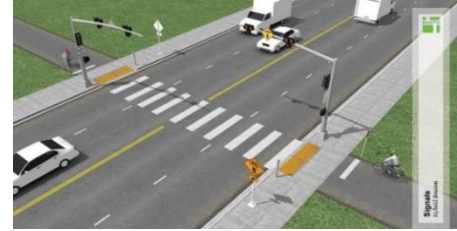
Figure 3: NACTO Intersection Schematic (Hybrid Beacon)
